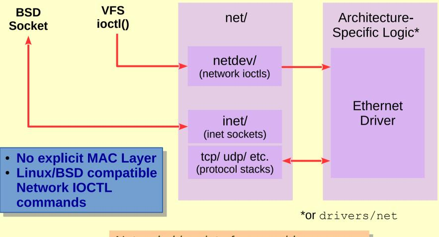
Network driver interface provides common Inteface between stacks and Layer2
