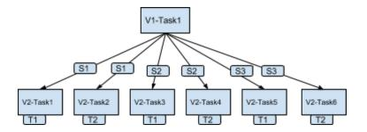
The first vertex will process the smaller input (S in example above) and send the inputs to a subset of of reduce tasks. For example input S1 is sent to Reducer1, Reducer 2. This would need a custom edge?
