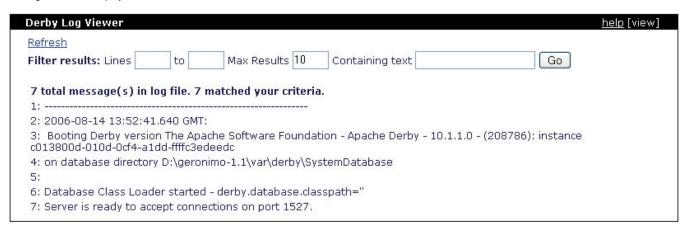
The **Refresh** link on the upper left corner will reset any filtering criteria you may have specified to the Geronimo Administration Console's defaults and will display the last 10 lines (if any) of the current Derby server log.
