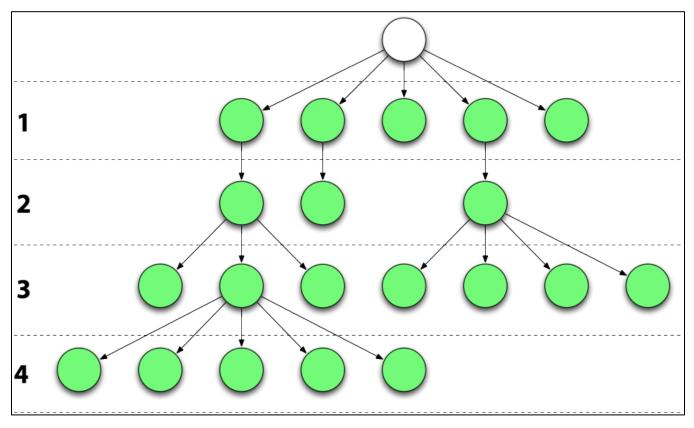
Each node in the graph represents a module in a multi-module build, the "levels" simply indicate the distance to the first module in the internal reactor dependency graph. Maven calculates this graph based on declared inter-module dependencies for a multi-module build. Note that the parent maven project is also a dependency, which explains why there is a single node on top of most project graphs. Dependencies outside the reactor do not influence this graph.
