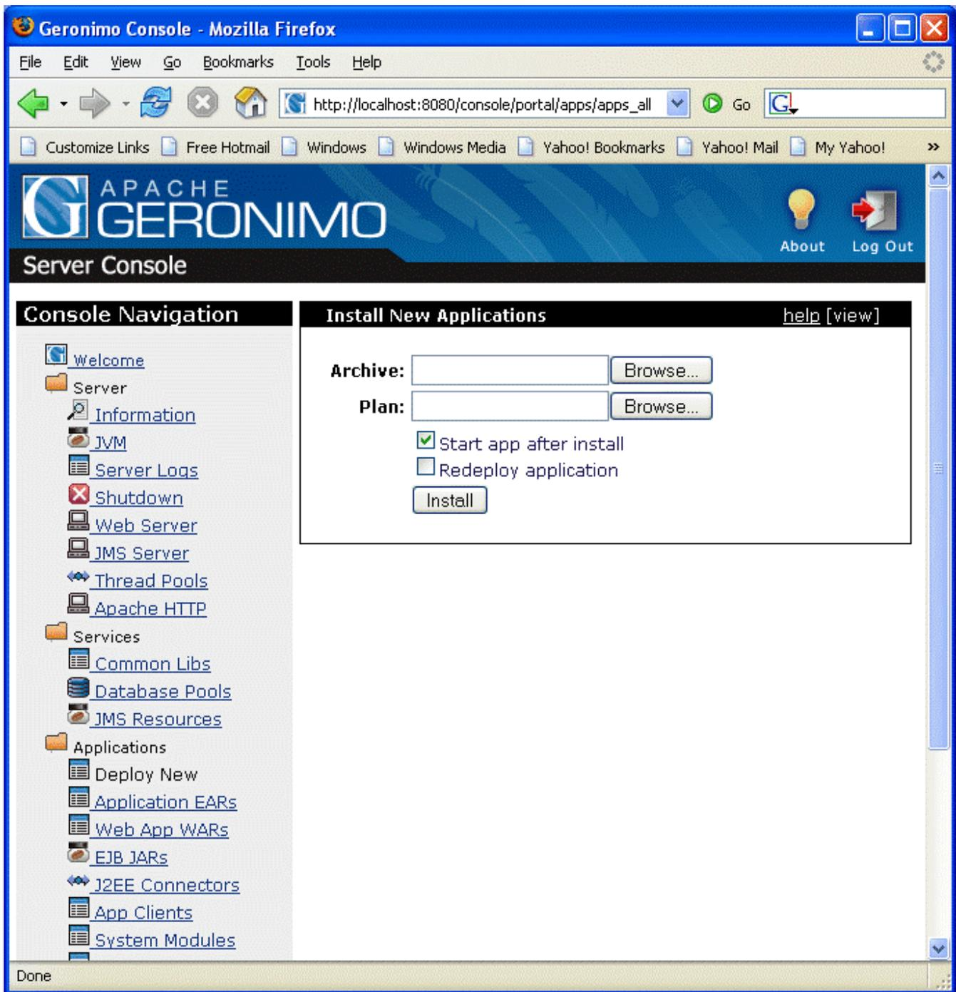
Then select and load the HelloWorld.war file into the **Archive** input box and click **install** button to deploy application in to the server. Once the application is successfully deployed, the screen will be updated with a successful deploy message. Before clicking the install button, make sure that the "Start app after install" checkbox is enabled.
