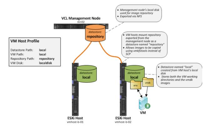
The diagram above shows a simple VCL configuration with 1 management node and 2 VMware ESXi hosts. Network storage is not used. The local disks on the VM hosts are used to store all of the files used by running VMs including the VM's working directory and the master vmdk image.
