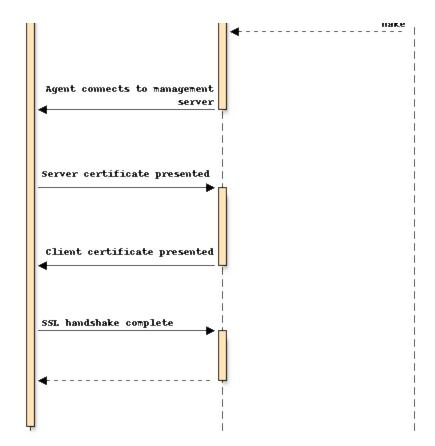
S3. SSL handshake and negotiations on connection/re-connection:
