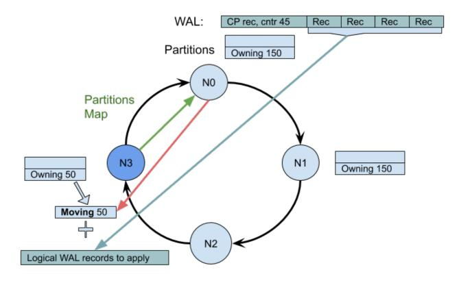
Coordinator observes older partition state and forces partition to moving state. Moving force is required to setup uploading newer data.
