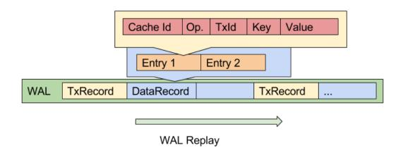
Data record includes list of entries (entry operations). Each operation has cache ID, operation type, key and value. Operation type can be
